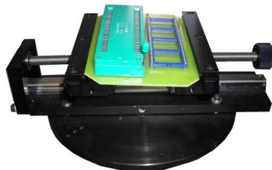
Packaged Part Holder can be opened and closed. It will hold large devices and small ones.
